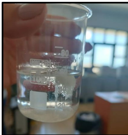
Figure a.1: Mixture of ethanol and PVP with increased PVP ratio.
